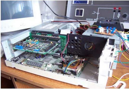
Figure 4 Hardware part of the acquisition system configured for monitoring of the electric solar energy parameter from solar panel output circuits
