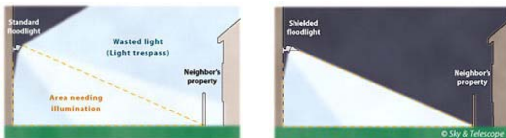
Figure 8 The difference of light distribution between standard floodlights and shielded floodlights [10]
