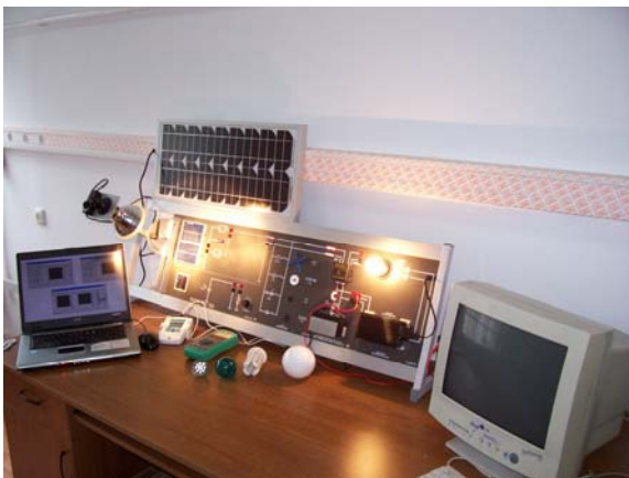
Figure 3 Experimental workstation for study of lighting system based on renewable energy
